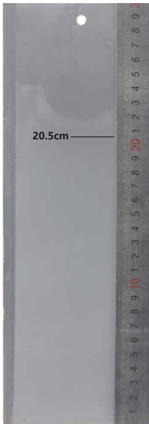
HTP-7000 series throwing power reach over 20cm by Ford method HTP-7000系列泳透力福特盒法达到20cm以上
